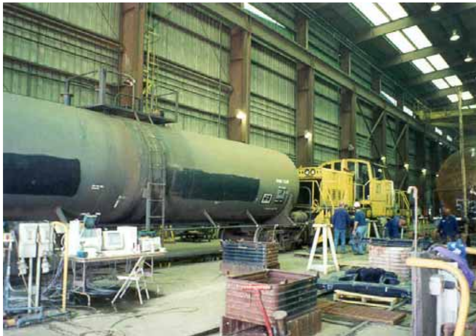
Figure 4.6 Switch Engine used to apply Draft Load to Bar Reinforced Tank Car
